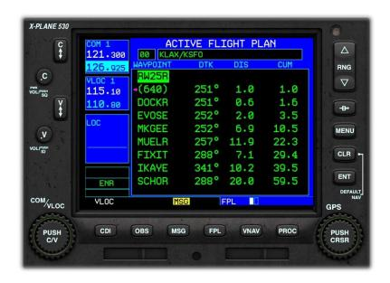
The chosen departure procedure is now converted to the individual waypoints it comprises. These appear in the appropriate order at the start of your flight plan.
