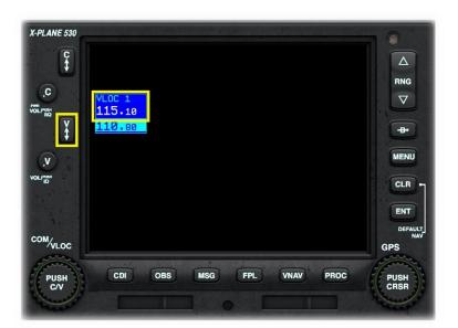
Click the VLOC (VOR / Localizer) Frequency Flip-Flop Key to swap the standby and active NAV frequency.
