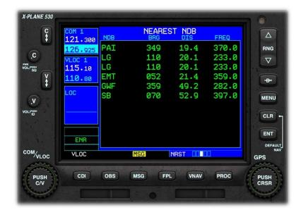
This Page displays the nearest NDB (Non-Directional Beacon) to your current location, together with the direct heading (bearing) to that NDB, the distance, and the frequency (for manually-tuned ADF devices).
