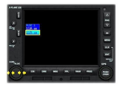
Click the CENTER of the Comm / VOR Localizer Rotary to highlight the standby NAV frequency.
