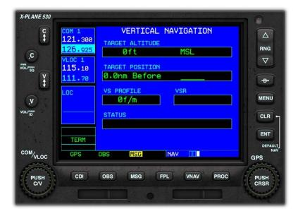
The Vertical Navigation (VNAV) Page provides the capability to designate a target altitude for a <u>single</u> waypoint in your flight plan. This feature is only active during the execution of a flight plan, or a "Direct To" instruction.
