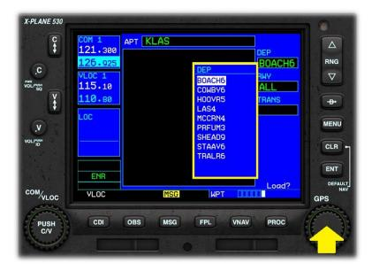
This Page displays supports the selection of the desired SID (Standard Instrument Departure) procedure for the airport of origin.
