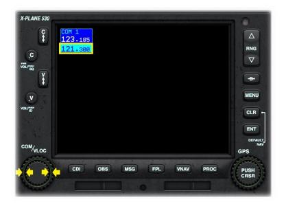
Click the CENTER of the Comm / VOR Localizer Rotary to highlight the standby COM frequency.
