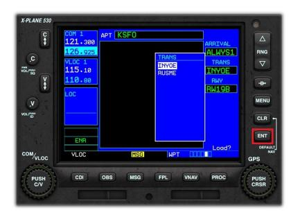
Click the GPS Inner Rotary at the 3 O'clock and 9 O'clock positions to select the desired transition waypoint.
