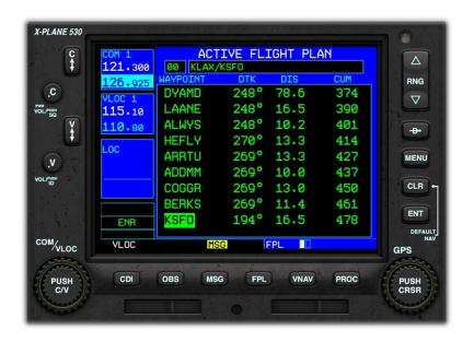
The chosen arrival procedure is now converted to the individual waypoints it comprises. These appear in the appropriate order at the end of your flight plan.
