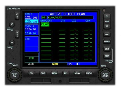
To create, update or delete waypoints in a flight plan, the cursor must be activated.
