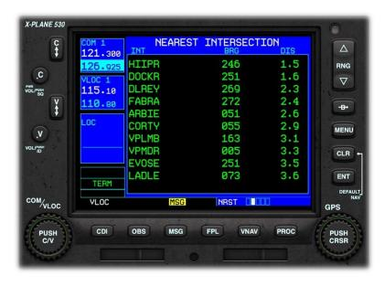
This Page displays the nearest intersection to your current location. An intersection is a virtual navigation fix, and is usually (but not always) the intersection of two VOR radials.
