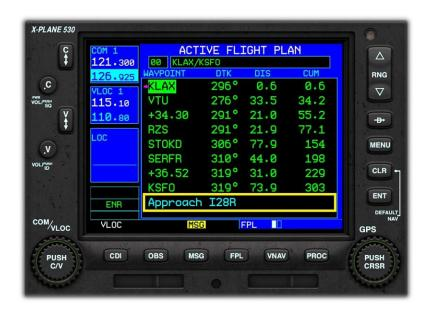
The chosen approach procedure is displayed in your flight plan, immediately after the destination airport.
