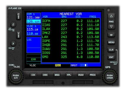
This Page displays the nearest VOR to your current location, together with the direct heading (bearing) to that VOR, the distance, and the frequency (for manually-tuned VOR receivers).
