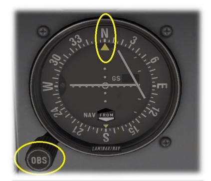
Using the OBS Rotary associated with the VOR/ILS Receiver on the instrument panel:
