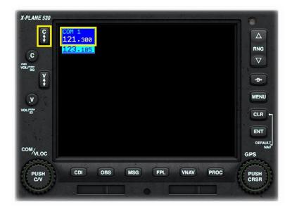
Click the Comm Frequency Flip-Flop Key to swap the standby and active COM frequency.
