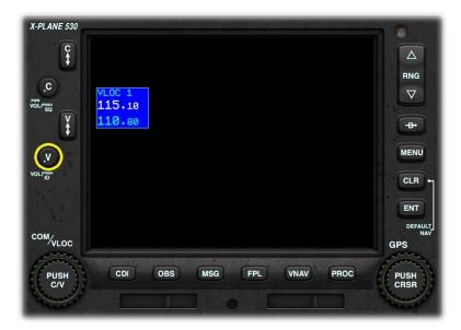
When the NAV frequency is tuned to a navigation aid that is within range, an audible Morse-Code identifier is available, to confirm the correct tuning.
