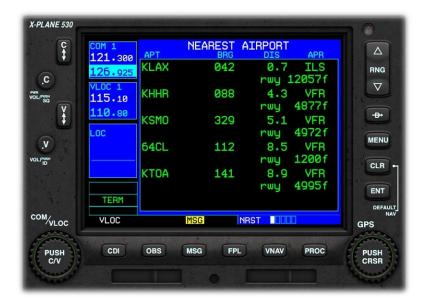
This Page displays the nearest airport to your current location, together with the direct heading (bearing) to that airport, the distance, the available approach-type (or VFR) and the length of the longest runway.
