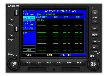
Click the FPL (Flight Plan) button to invoke the Flight Plan Page (1 of 2).
